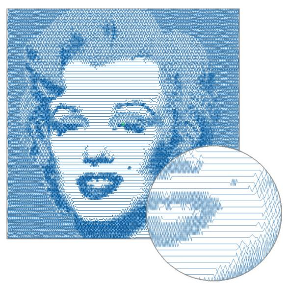
DENSITY MODE: The height of the zig-zags is constant; the density of the pattern, i.e. the distance between the points reflects the gray scale.
